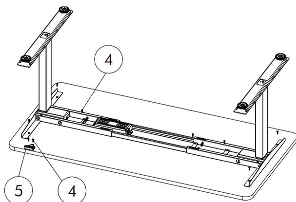
STEP 6: Mount the frame to the table top with 7 ST4.8\*20 tapping screws and the handset with 2 ST4.8\*20 tapping screws. Tighten the screws.
