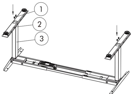
STEP 4: Ad the feet on to the columns and fasten each with 2 screws. Tighten the screws.
