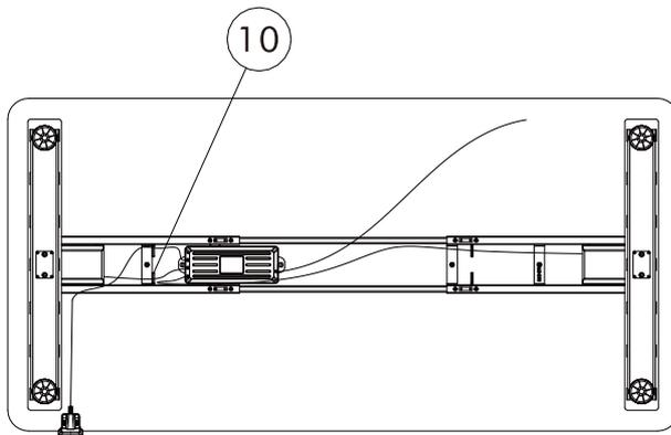
STEP 8: Stick the four cable clips into the frame, ensure that the cables are placed properly.
