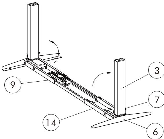
STEP 2: Raise the columns and tighten the screws to the end rail through the frame. Start with the left column followed by the right column.
