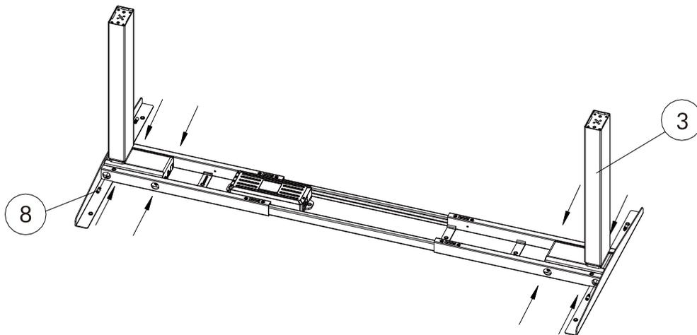
STEP 3: Ad 8 M6\*10 hexagon screw through the frame into the motor house of the columns. Tighten the screws.
