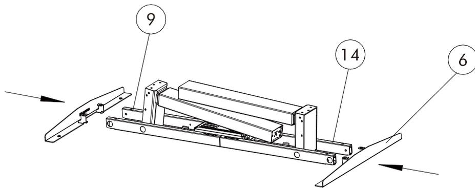
STEP 1: Ad both end rails to the frame.
