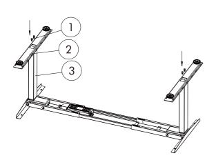
STEP 4: Ad the feet on to the columns and fasten each with 2 screws. Tighten the screws.
