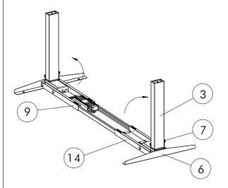
STEP 2: Raise the columns and tighten the screws to the end rail through the frame. Start with the left column followed by the right column.
