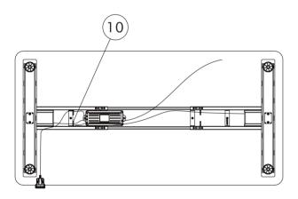
STEP 8: Stick the four cable clips into the frame, ensure that the cables are placed properly.
