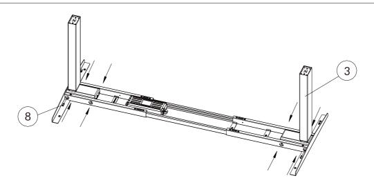
STEP 3: Ad 8 M6\*10 hexagon screw through the frame into the motor house of the columns. Tighten the screws.
