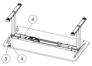
STEP 6: Mount the frame to the table top with 7 ST4.8\*20 tapping screws and the handset with 2 ST4.8\*20 tapping screws. Tighten the screws.
