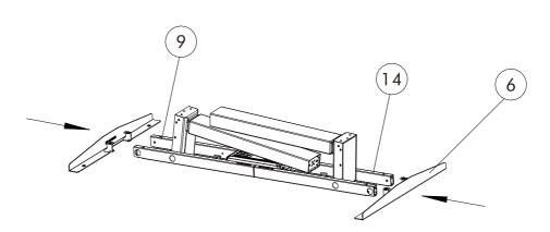
STEP 1: Ad both end rails to the frame.
