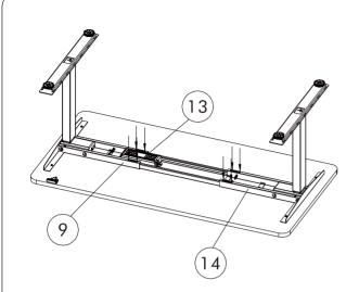
STEP 7: Tighten all 8 screws in the frame.
